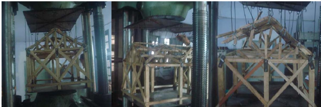
Fig 6: Experimental setup under suction force in UTM
